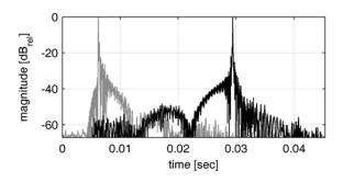
Figure 6-5. Impulse responses of compensated HpTFs. Left/grey: using an LMS filter designed to exhibit minimum phase (acc. to [20]), right/black: using an LMS filter without constraints to filter phase designed to best approximate the (linear phase) target function after compensation.
