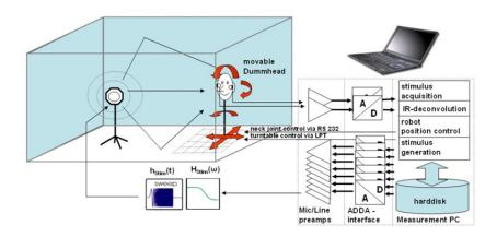
Figure 2-3. Complete setup for the measurement of room impulse responses in multiple degrees of freedom.
