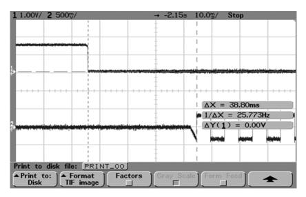
Figure 9-1. Screenshot from minimum TSL measurement, upper trace: falling edged indicates a starting tracker movement, lower trace: output of the convolution. After a fade-in of the duration of one audio block size an alternating square wave is rendered.
