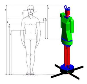
Figure 2-2. Anthropometric measures and the resulting 3D-CAD drafts of the modular torso.
