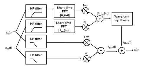
Figure 11-3. Block diagram of TB-SI algorithm: Low frequency information is derived from continuously crossfading between the two microphones' signals  $x_n(t)$  and  $x_{nn}(t)$  closest to the respective ear. High frequency information is derived through interpolation of short-time magnitude spectra and phase reconstruction during waveform synthesis (after [5]).
