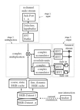
Figure 5-5. Simplified block diagram of rendering application.
