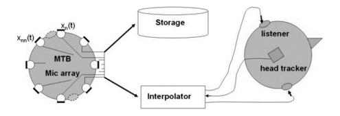
Figure 11-1. Sketch of MTB reproduction principle: A head tracker determines the position of the listener's ears. The signals of the two microphones which are closest to the position of an ear,  $x_n(t)$  and  $x_{nn}(t)$ , are selected and ear signal are constructed by interpolating between these microphone signals while continuously following the head orientation. Ear signals can be constructed instantaneously or off-line from stored MTB recordings (drawing after [5]).
