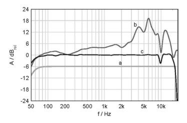
Figure 7-3. Individual linearization of BK211 without repositioning: (a) desired target response (shifted by -6 dB), (b) HpTF displayed with 1/6 octave smoothing, (c) linearized HpTF displayed with 1/6 octave smoothing. The compensation filter was derived from case (b) using a parametrical filter regularized LMS-inversion.
