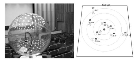
Figure 11-4. Left: Virtual MTB mounted on a remotely rotatable basement in the middle of a lecture hall. Notice the singular microphone mounted in the plastic sphere. Right: Sketch of loudspeaker arrangement used for impulse response measurements with the virtual MTB array (distances are given relative to the virtual MTB's location; circles indicate multiples of the critical distance which was 3.17 m).
