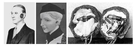
Figure 1-2. Left: "Oscar", artificial head and torso applied for binaural transmissions of musical concerts by Bell Laboratories (Hammer and Snow, 1932). Middle: Display mannequin with microphones placed in rudimentary outer ears used by de Boer and Vermeulen (1939). Right: Inner view of an early artificial head molded from a human corpse's head by Alvar Wilska (1938) in the course of his doctoral thesis.
