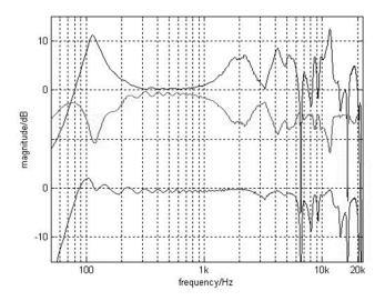
Figure 5-3. Frequency response of STAX SR 202, frequency response of inverse LMS filter (N=1024) with frequency-dependent regularization, calculated frequency response after compensation (from upper to lower).
