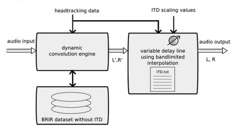
Figure 8-4. Schematic depiction of the signal flow in dynamic binaural synthesis with real time individualization of the ITD.
