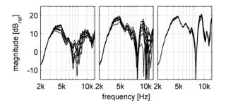
Figure 6-2. Ten transfer functions of an artificial ear measured with Knowles FG 23329 and EAR II foam plug (left), UVEX foam plug (middle), and novel silicone earplug (right), when plugs were reinserted between each measurement (from [18]).
