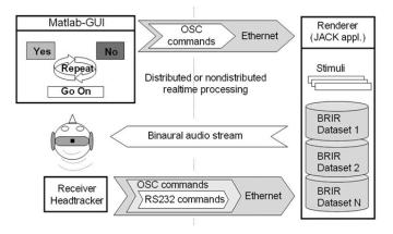
Figure 5-6. Flow diagram of control and audio data in the rendering process.
