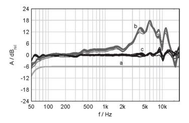
Figure 7-2. Individual linearization of BK211 with repositioning between measurements: (a) desired target response (shifted by -6 dB), (b) 11 measured HpTFs displayed with 1/6 octave smoothing, (c) linearized HpTFs displayed with 1/6 octave smoothing. The compensation filter was derived from the complex average of case (b) using a high-shelve filter regularized LMS-inversion.
