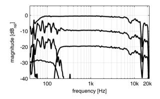
Figure 6-6. Magnitude spectra of compensated HpTF (frequency domain LMS inversion with highpass-regularization) measured at a test subject's right ear. Curves top down: 1) full range head-phone reproduction, 2) sum response of 2-way reproduction, 3) 2-way reproduction, subwoofer and headphones shown separately, 4) near field response of subwoofer (all curves 1/24th octave smoothed, 10 dB offsets for clarity).
