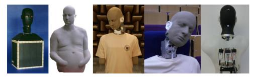
Figure 1-4. Artificial heads or HATS devices that may move their head in one (photo no. 1: rotatable artificial head [Neumann Ku100] used by Mackensen [2004]; photo no. 2: HATS built by Moldrzyk [2002]) or more degrees of freedom (photos no. 3 and 4, HATS FABIAN, courtesy of the author, photo no. 5, rear view of HATS by Hess and Weishäupl, [2014]).
