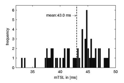
Figure 9-2. Distribution of measured minimum TSL values, the broken line indicates the mean value (resulting true end-to-end latency as realized in the listening test is shown including additional 70 samples of delay from BRIR datasets and headphone compensation).
