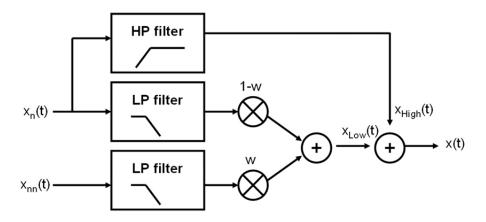
Figure 11-2. Block diagram of TB-NM algorithm: Low frequency information is restored from continuously crossfading between the two microphones' signals  $x_n(t)$  and  $x_{nn}(t)$  closest to the respective ear. High frequency information is restored by switching between the respective nearest microphone signals, e.g., here  $x_n(t)$  (after [5]).
