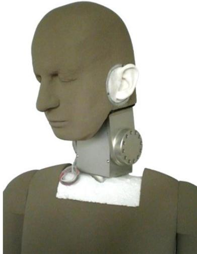
Figure 2-1. Close-up view of the FABIAN dummy head with uncovered neck joint.
