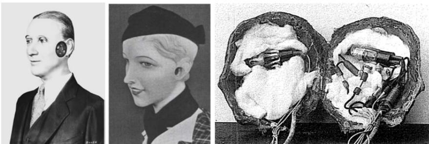
Figure 1-2. Left: “Oscar”, artificial head and torso applied for binaural transmissions of musical concerts by Bell Laboratories (Hammer and Snow, 1932). Middle: Display mannequin with microphones placed in rudimentary outer ears used by de Boer and Vermeulen (1939). Right: Inner view of an early artificial head molded from a human corpse's head by Alvar Wilska (1938) in the course of his doctoral thesis.
