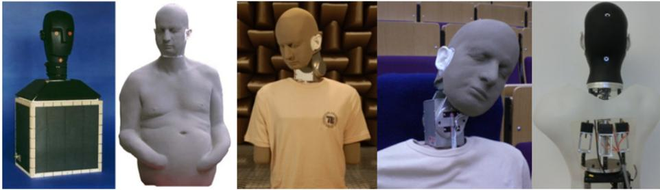
Figure 1-4. Artificial heads or HATS devices that may move their head in one (photo no. 1: rotatable artificial head [Neumann Ku100] used by Mackensen [2004]; photo no. 2: HATS built by Moldrzyk [2002]) or more degrees of freedom (photos no. 3 and 4, HATS FABIAN, courtesy of the author, photo no. 5, rear view of HATS by Hess and Weishäupl, [2014]).
