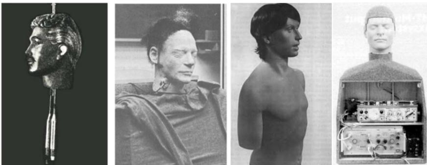
Figure 1-3. From left to right: (1) Mould of a display mannequin’s head with partly mechanically reworked outer ears (Damaske and Wagener, 1969). (2) Artificial head as a combination of gypsum and rubber molds of a real individual (Kürer, Plenge und Wilkens, 1969). (3) KEMAR (Knowles Electronic Manikin for Acoustic Research) with a wig (Burkhardt and Sachs, 1975). (4) Prototype of Genuit’s artificial head recording system intended for acoustic measurement purposes (Genuit, 1981).
