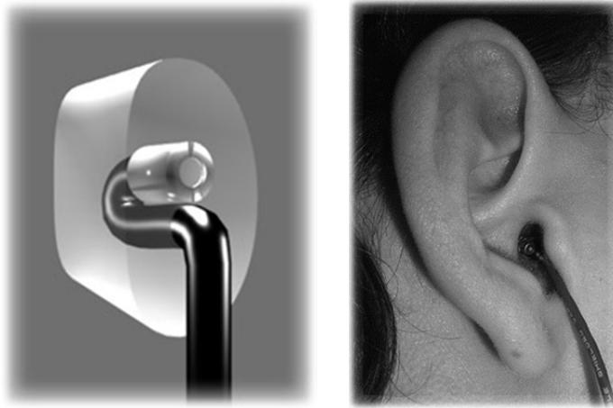
Figure 6-1. Custom-built silicone earplug. Left: CAD model, right: inserted into a subject's ear (from [18]).
