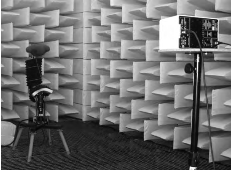
Figure 7.14: Setup used for the HRTF-measurements.
