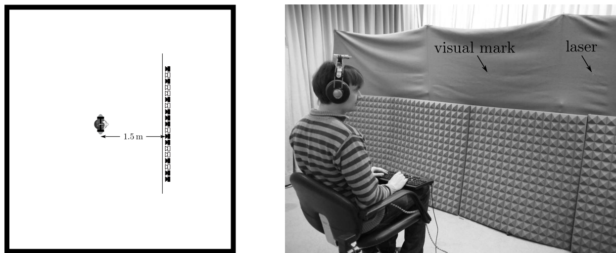
Fig. 1: Sketch of the experimental setup (left) and picture of a subject during the experiment (right). Only the filled loudspeakers were used in the first experiment. The light in the room was dimmed during all experiments.
