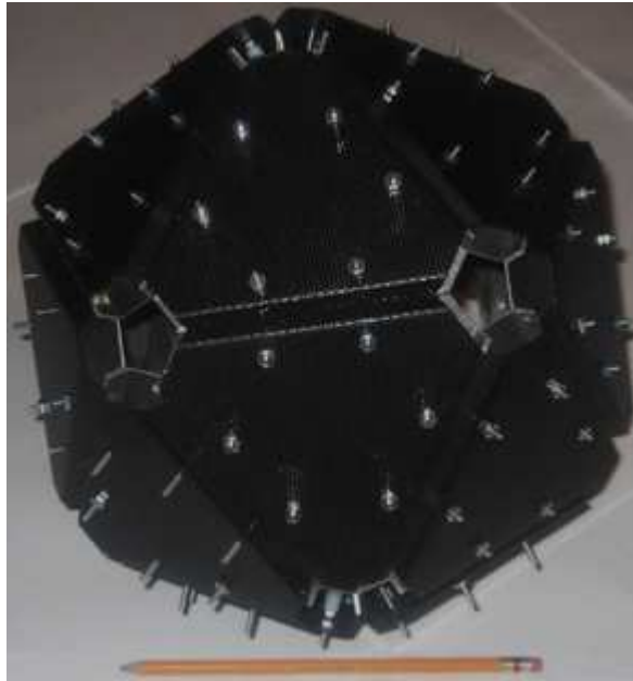
Figure 1.4: The 120 independent element spherical loudspeaker array developed at Berkeley’s CNMAT. ( Photo from CNMAT , http://www.cmat.berkeley.edu/Research/AES2006/speakerarray/icosaspeakers.htm )
