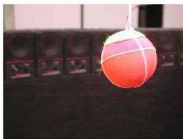
Figure 4.11: The sound installation Scratch during the Linux Audio Conference. In the ball are accelerometers to measure the movement of the ball, which influences the sound installation ( photo by Frank Neumann ).
