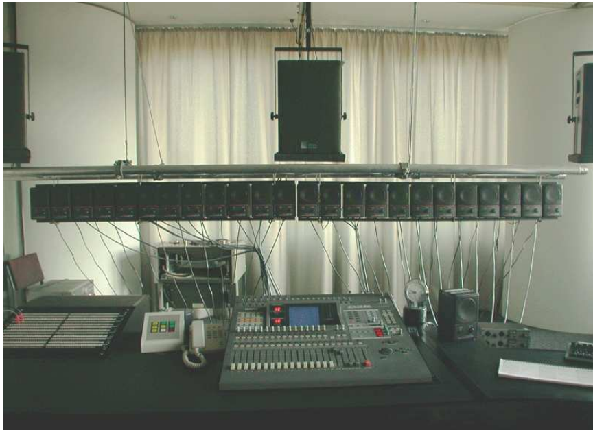
Figure 3.1: The 24 FOSTEX loudspeakers in a WFS setup in the electronic studio of the TU Berlin ( photo: Folkmar Hein ).
