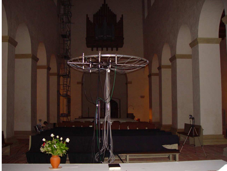
Figure 4.2: A circular recording array, as developed at the TU Delft [HSdVB03]. Here in action for a recording in the Liebfrauenkirche in Halberstadt, Germany (Photo by Bernhardt Albrecht).
