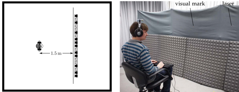
Figure 4.3: Sketch of the apparatus in the listening room (left) and a listener during the experiment (right). Only the loudspeakers marked in black were used in the experiment. Note that the room was dark during the experiment.
