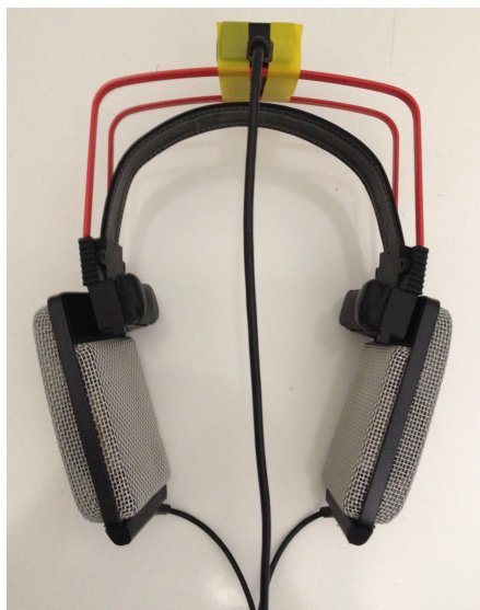
Figure 3.11: AKG K1000 extra-aural headphones with Razor AHRS head tracker mounted on the rim.
