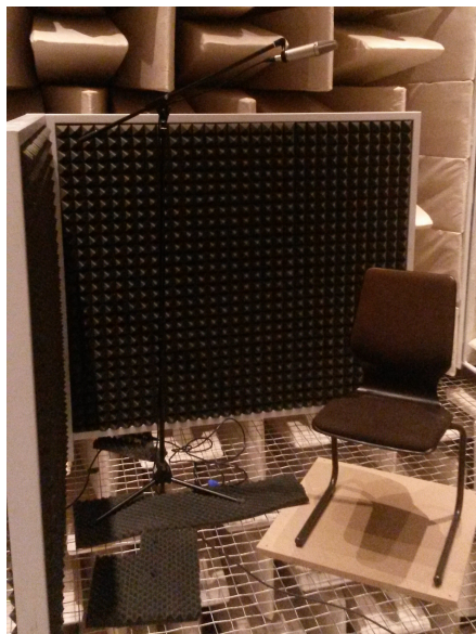
Figure 3.15: Recording setup of the violin player in the anechoic chamber for the comparative test of different replication algorithms.
